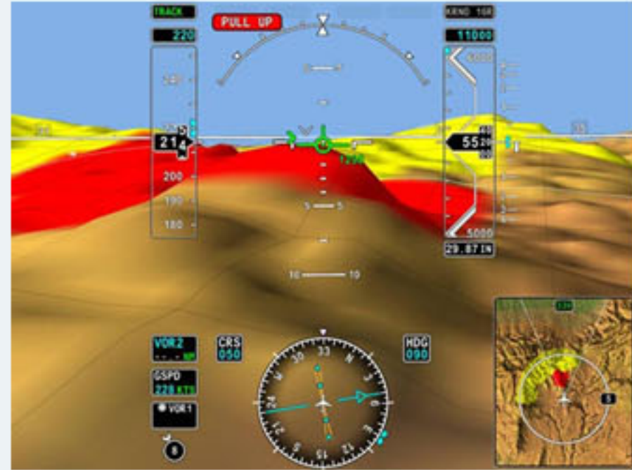
Honeywell Aerospace's Synthetic Vision System uses an Integrated Primary Flight Display to show pilots towers, rising terrain and other obstacles at any time (day or night) and in any type of weather. Credit: Honeywell Aerospace.
