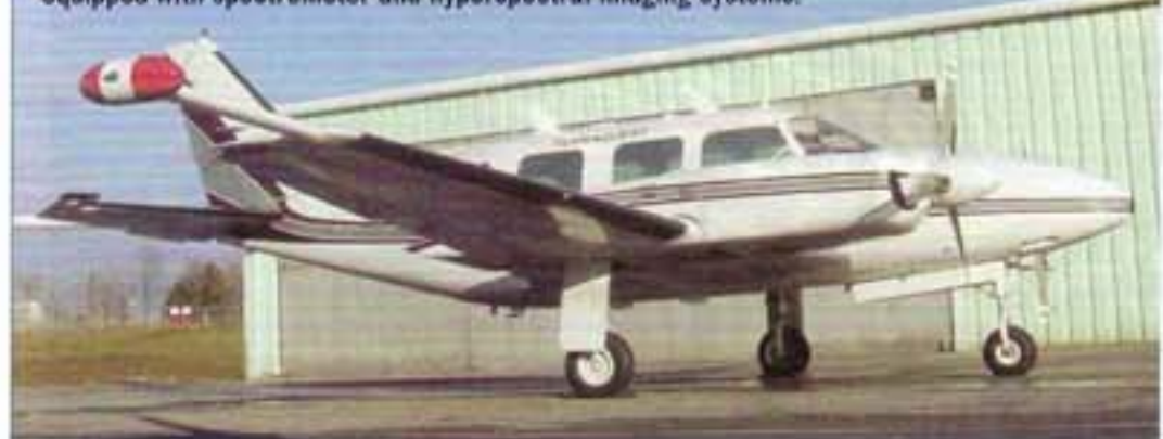
The Terraquest Ltd. Piper PA-31 Navajo was modified for magnetic survey and can also be equipped with spectrometer and hyperspectral imaging systems.
